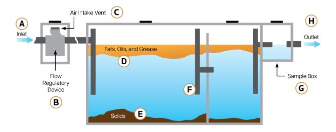
Flow from undersink grease traps or directly from plumbing fixtures enters the greaseA interceptor. The Uniform Plumbing Code (UPC) requires that all flow entering the interceptor must enter through the inlet pipe.
