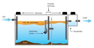
A grease interceptor should be checked and maintained to ensure that it is working properly. Backups, odors, and drainage problems are signs that the grease interceptor is not functioning as it should. See OC San's Fact Sheet for Grease Interceptors for specific tips on proper maintenance of grease interceptors.
